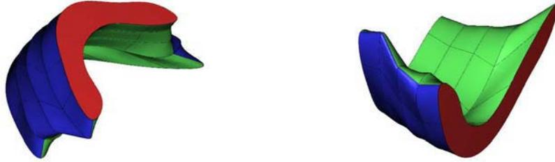
**Fig. 4.** Loading and constraints on surface regions. Blue: exterior surface, green: interior surface, red: anterior and posterior surfaces.
